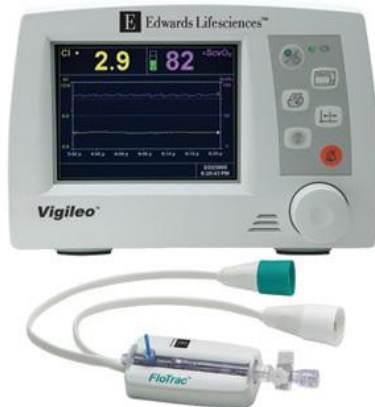
Figure 1 The Vigileo monitor and the FloTrac sensor cuff (40)
