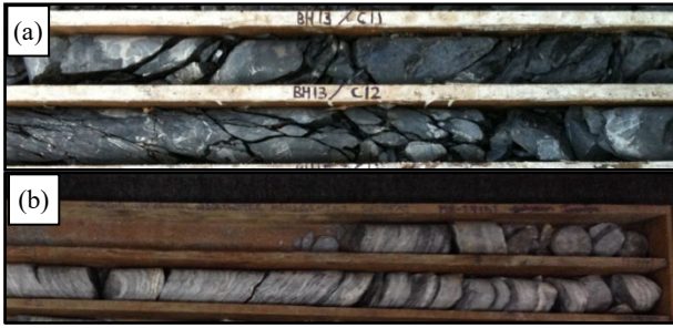
Fig. 1. Rock cores demonstrating very low RQD upon retrieval from highly weathered Tuang Formation for lithological units of (a) phyllite; and (b) shale. (Ong and Choo, 2018)
