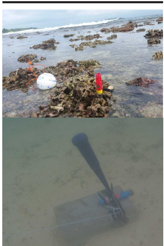
Figure 3. Example RBR monitoring station over the flat reef showing the aerial exposition during low tide (left) and example of current monitoring station (right).
