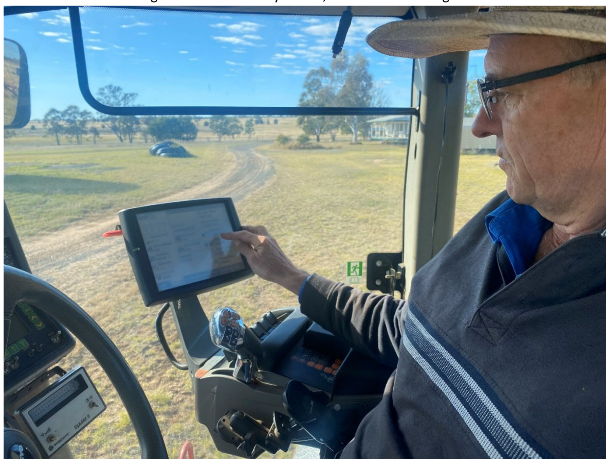
Figure 2: Peter Thompson operating GPS and autosteer on the Quadtrac tractor.
