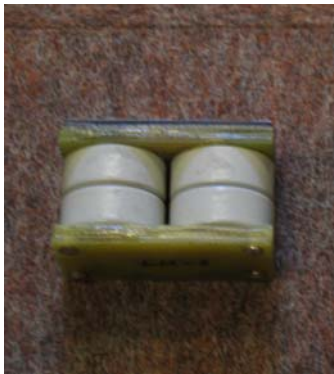
(a) HFCT over view
