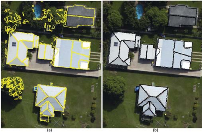
Fig. 3. Removal of false planes: (a) all plane boundaries from the Aitkenvale data set and (b) refined plane boundaries.
