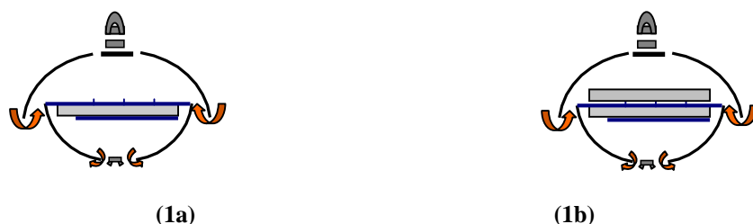
Figure 1: PUF disks housed in passive sampling chamber with both 1-PUF (1a) and 2-PUF (1b) configurations.
