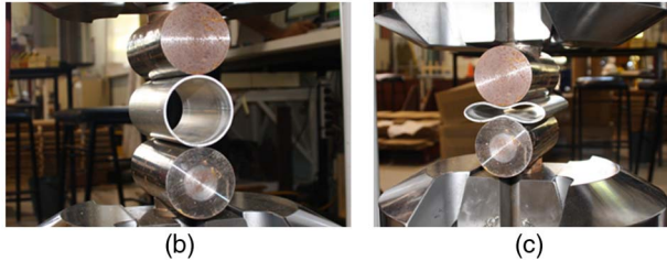
Fig. 6. (a) Ring squash test results for single pipe ( 60 \times 2 mm); (b) Collapse State 1; (c) Collapse State 2
