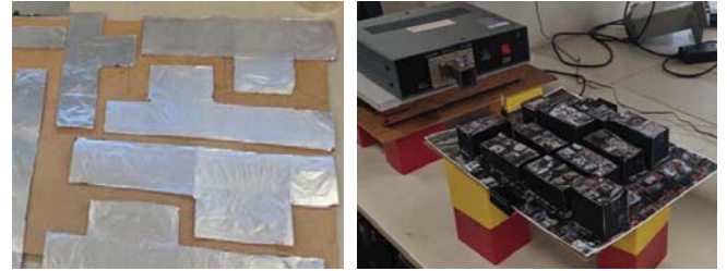
Fig. 6. Set up including Gunn oscillator, model city, antenna, detector (not visible) and voltmeter (not visible).
