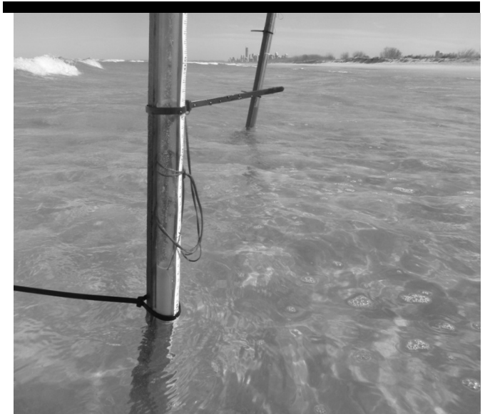
. Stilling Well shows the long wave water level fluctuation 2Figure
