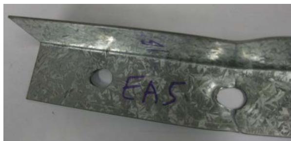
Figure 5 Net section tensile rupture of an angle brace bolted at one leg
