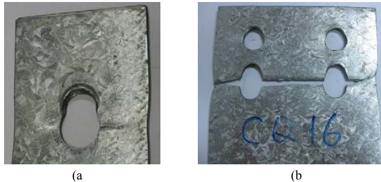
(a) (b) Figure 1 Net section tensile ruptures in flat sheets
