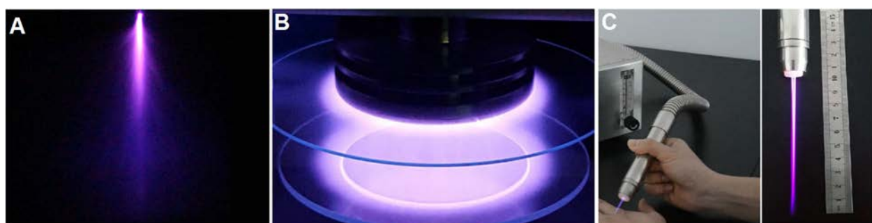
Fig. 2 Typical measures to produce cold plasma at atmospheric pressure include corona (a), DBD (b), and APPJ (c)
