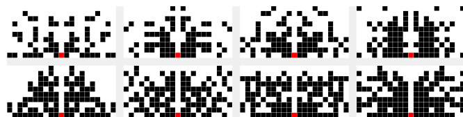
Figure 7: Sample population using a Gaussian distribution around the feed point. The approach produces some continuous structures around the feed point with many disconnected elements around them. A possible downside will be the lack of patches in the corners far from the feed point, leading to a potential bias in the search.
