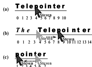
Figure 2: The PRA effect (the telepointer tracks the reference character “p”). (a) The initial state; (b) The state after executing an insert; and (c) The state after executing a delete.
