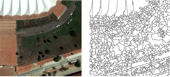
Fig. 1. An example of watershed segmentation. The left hand is the original image. The right hand shows the corresponding watershed segmentation results.
