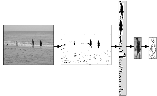
Fig. 2. Object detection and segmentation process shown from left to right. The original image, the image after applying the moving average algorithm, segmented images, image component containing the grey-scale image, and the edge detected image (not to scale).
