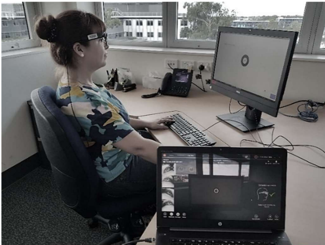
Figure 3.1 A participant wearing an eye-tracker and the calibration process
