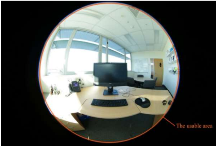
Figure 3.4 The captured LDR image and the usable area for making the HDR image
