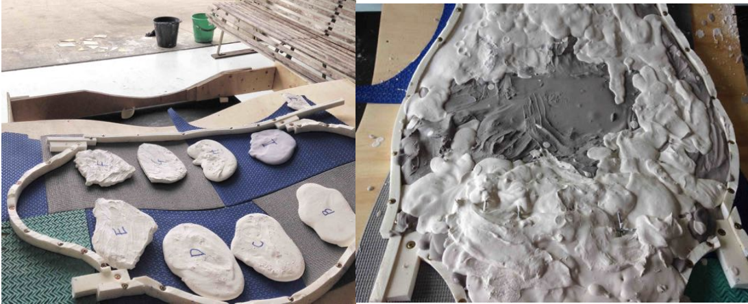
Fig.44 Coronas 2016 with precast elements arranged face down on composition of patterned surfaces prior to inserting the linoleum pieces. The curved armature of plywood is visible upper centre and the washed lino pieces are drying on the ground near the buckets. The amalgamation is completed with several pours of pigmented modified gypsum.
