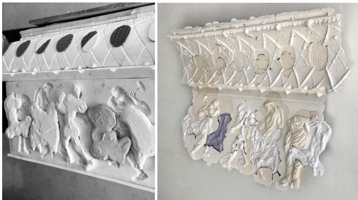
Fig.41 left: Cornice Frieze 2015 mould with precast characters positioned prior to casting and right: Cornice Frieze 2015.
