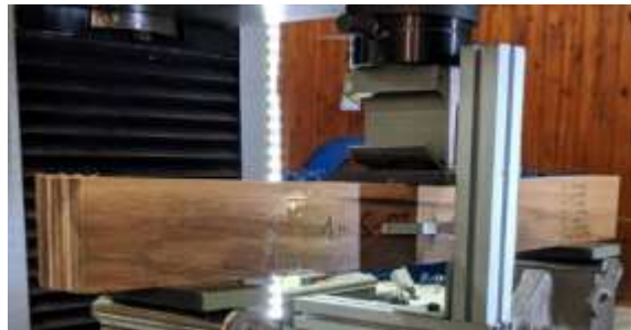
Fig. 7. Testing configuration for longitudinal shear strength
