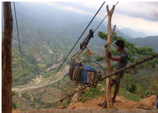
1b. Goods loaded in first trolley in the uphill station being transported to bottom station
