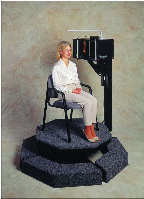
Fig. 1. The Cyberware Head & Face Colour 3D Scanner [9] and the scanning process. Two of the lamps are installed on the scanner's head to provide light sources for texture acquisition.
