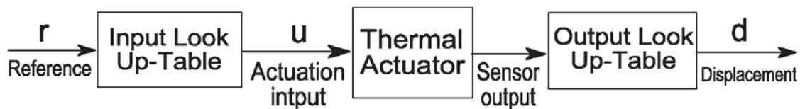
Figure 15 Block diagram of the open-loop control system including input and output look up tables, reference, electrothermal actuator and sensor. [39]
