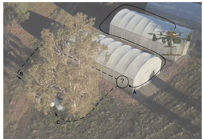
Fig. 1. Unmanned aerial vehicle (UAV) navigating in environments under uncertainty and partial observability. A small UAV with autonomous decision-making should be able to plan sequential sets of actions for optimal navigation trajectories, despite limitations from imperfect sensor data.
