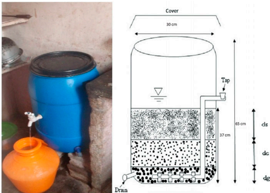
Figure 1. The Safe Water Treatment device operating inside a participant's home (left), and a cross-sectional diagram of the filter technology (right).
