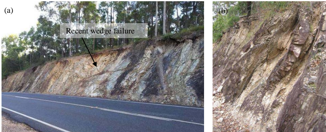
Figure 1. The study area: a) a rock slope comprised of argillite and greywacke of the Neranleigh-Fernvale Beds; b) bedding of the argillite.
